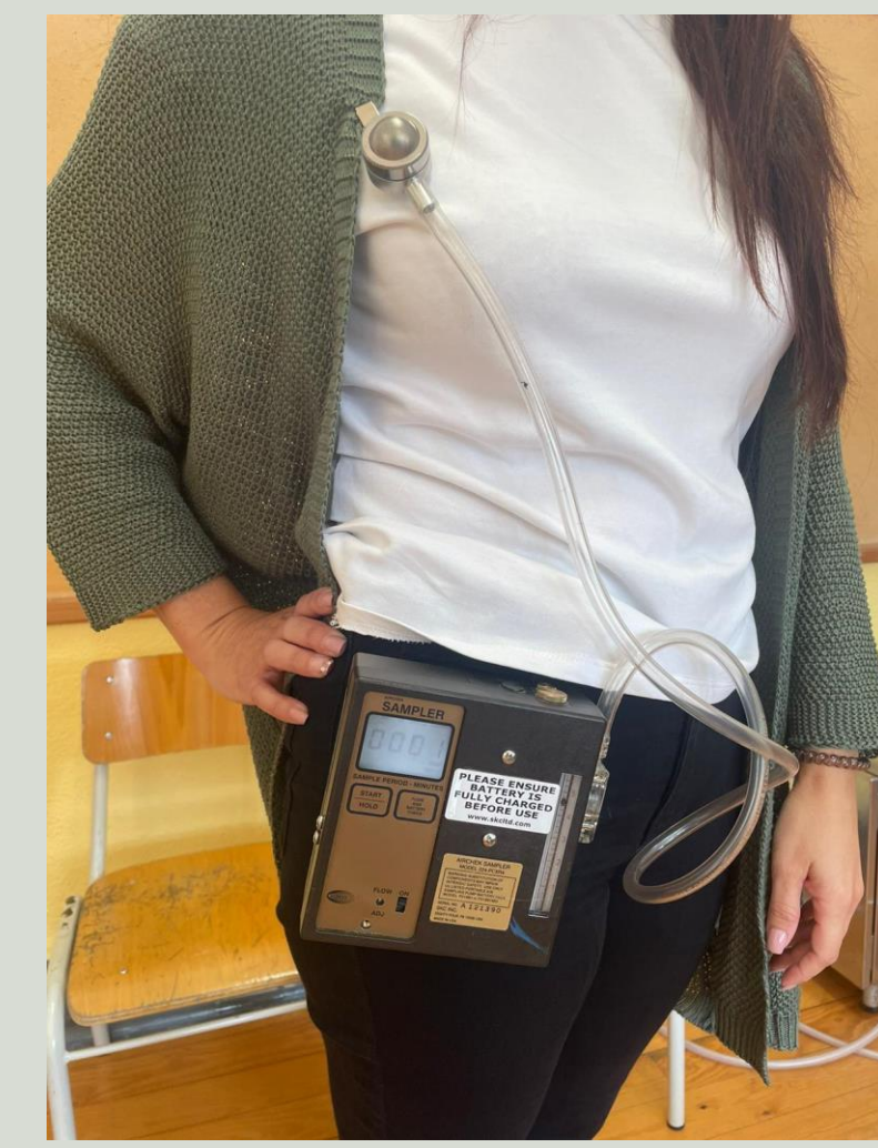
SKC Button sampler with Polycarbonate filter (2h at 4L/min)
